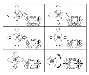
As shown in the above figure, in CF Mode (the bottom four LED lights keep flashing quickly) No matter where the aircraft locates(the red light is the onward direction), now the position of the remote controller is the rear of the aircraft. At this time, push the direction lever down, the aircraft will come back, and push the direction lever up, the aircraft will fy far away.
